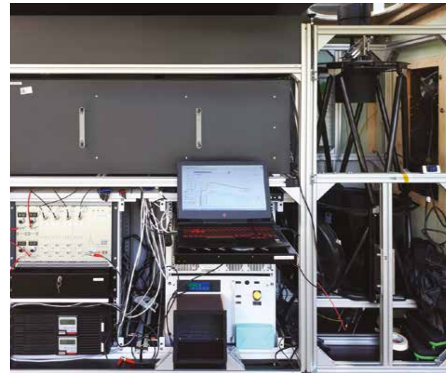
↓ Interior setup of the lidar system
